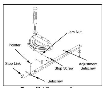
Figure 30. Miter gauge diagram
